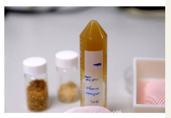
Pollen-derived ink (in the tube) is able to hold its shape when deposited onto a surface, making it a viable alternative to current inks used for 3D printing in the biomedical field (Credit: NTU Singapore)
